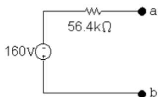
P 4.77  $V_{Th} = 0$ , since circuit contains no independent sources.
