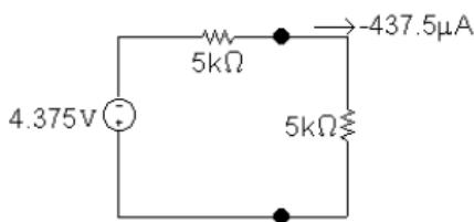
$$p_{\text{max}} = (-437.5 \times 10^{-6})^2(5000) = 957 \mu\text{W}$$
